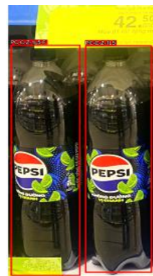
Figure 4. Detection Results After Applying the NMS Algorithm
