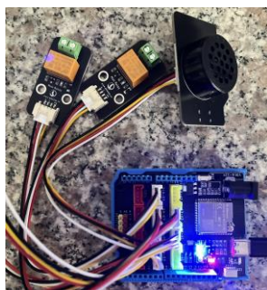
Figure 11. When no one is inside, the led on the board is green
