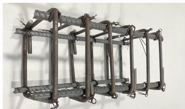
Figure 2. Geometry and reinforcement details of the reinforced concrete column specimen
