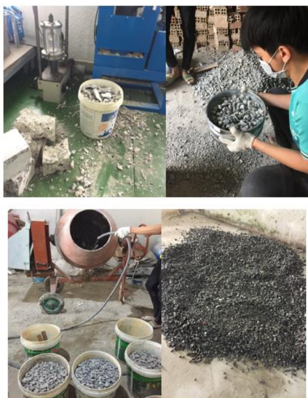
Figure 1. Collection and processing procedure of RCA
